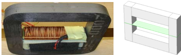
Fig.8. Non-standard SST used for experiments (left) and its simplified version in 3D FEM calculations (right)
