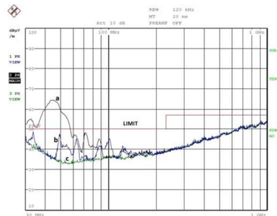
Fig. 10. Emission of radiated disturbance power supply for power  $P_{out1}$  with vertical antenna setting, the curve a - wires unshielded, curve b - shielded cables, curve c - background level
