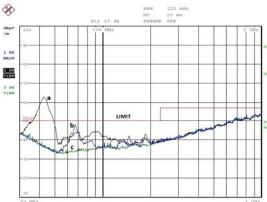
Fig. 12. Emission of radiated disturbance power supply for power  $P_{out2}$  by a horizontal antenna setting, the curve a - wires unshielded, curve b - shielded cables, curve c - background level
