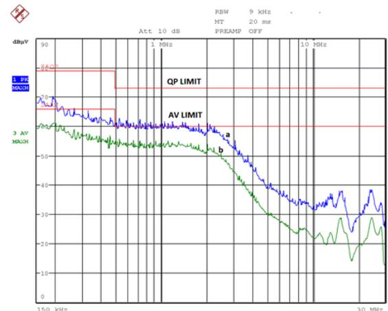
Fig. 17. Emission of conducted disturbances the power supply for the power  $P_{out2}$ ; curve a - peak detector PK, b - average detector AV, limits for listeners QP and AV
