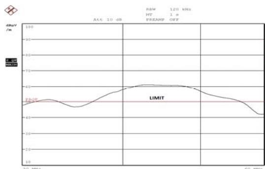
Fig. 11. Emission of radiated disturbance power supply for power  $P_{out1}$  on the vertical setting of the antennas and cables unshielded - the measurement verification detector QP
