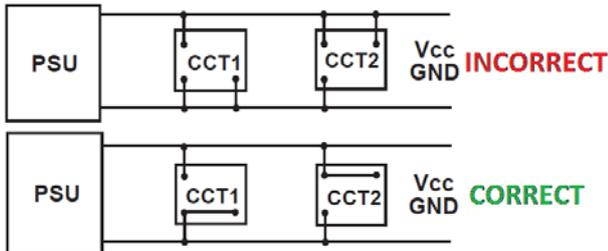
Fig. 5. Ways of carrying bus rails in multi-module electronic devices
