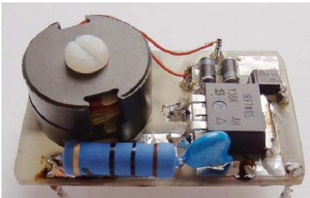
Fig. 7. General view of the model impulse power supply
