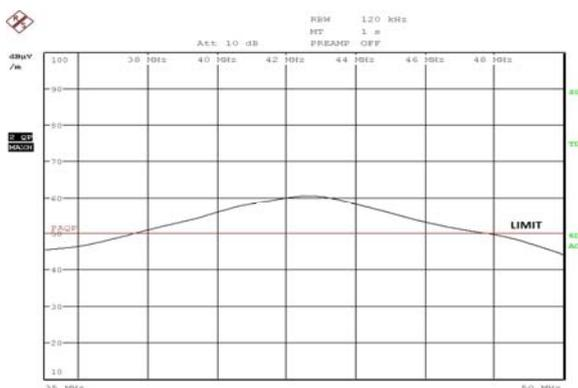
Fig. 13. Emission of radiated disturbance power supply for power  $P_{out2}$  with horizontal set antenna and cables unshielded - the measurement verification detector QP
