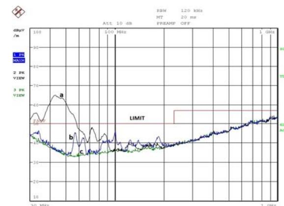
Fig. 14. Emission of radiated disturbance power supply for power  $P_{out2}$  with vertical antenna setting, the curve a - wires unshielded, curve b - shielded cables, curve c - background level
