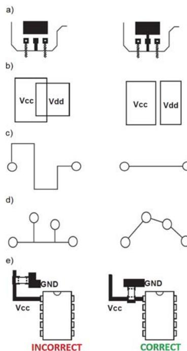
Fig. 4. Solutions used in the printed circuit boards of power supplies
