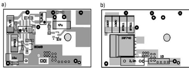
Fig. 6. View of two-sided printed circuit board power supply size 42x26 mm a) BOTTOM side; b) From TOP page
