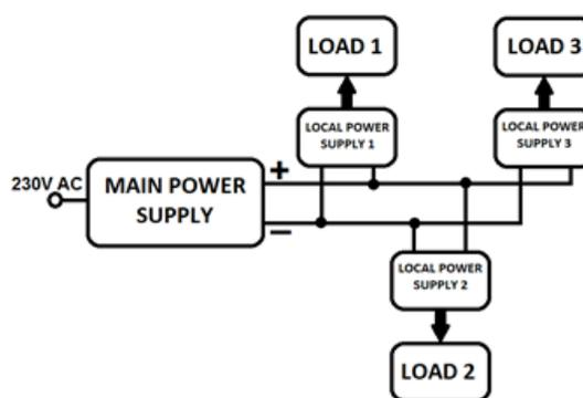
Fig. 1. Distributed architecture power supply system (DPS)
