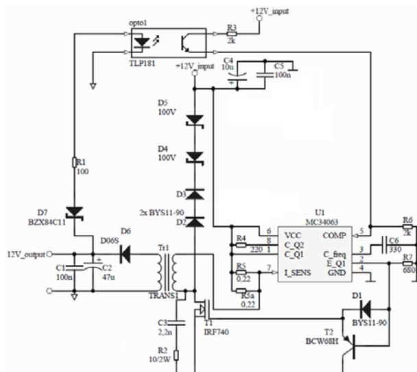
Fig. 3. Schematic diagram of the switching power supply with galvanic isolation
