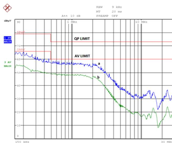
Fig. 16. Emission of conducted disturbances the power supply for the power  $P_{out1}$ ; curve a - peak detector PK, b - average detector AV, limits for listeners QP and AV
