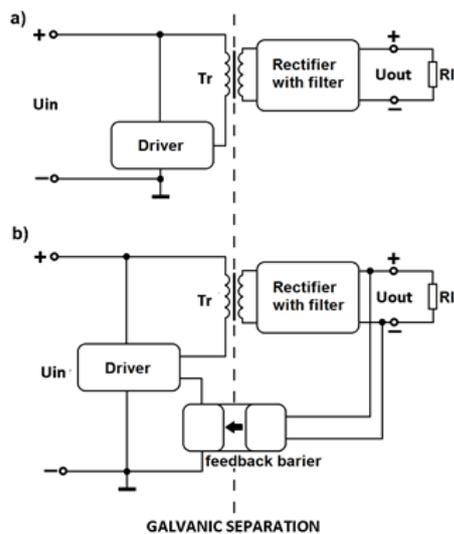
Fig.2. Basic switch mode power supplies settings; a) without stabilized output voltage; b) with stabilized output voltage
