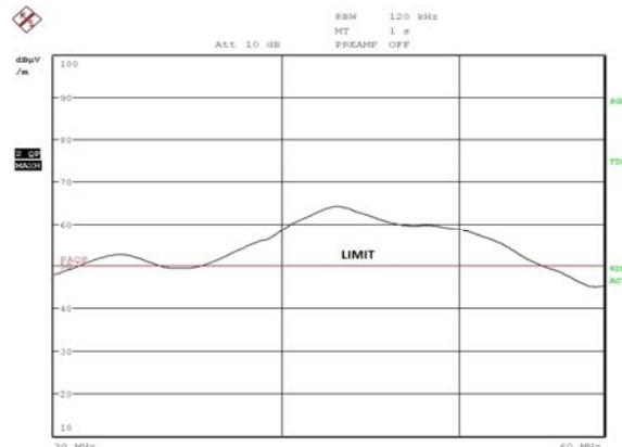
Fig. 15. Emission of radiated disturbance power supply for power  $P_{out2}$  on the vertical setting of the antennas and cables unshielded - measurement of the QP detector verification
