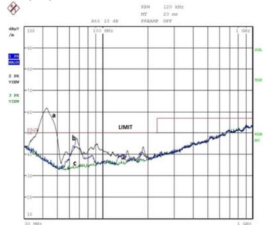
Fig. 8. The emission of radiated disturbance power supply for power  $P_{out1}$  by a horizontal antenna setting, the curve a - wires unshielded, curve b - shielded cables, curve c - background level
