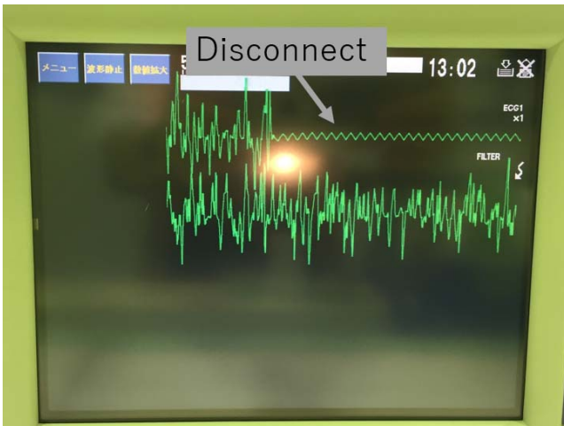
Fig.8. Disconnection of wireless medical telemetry system induced by electromagnetic noise from LED lamp
