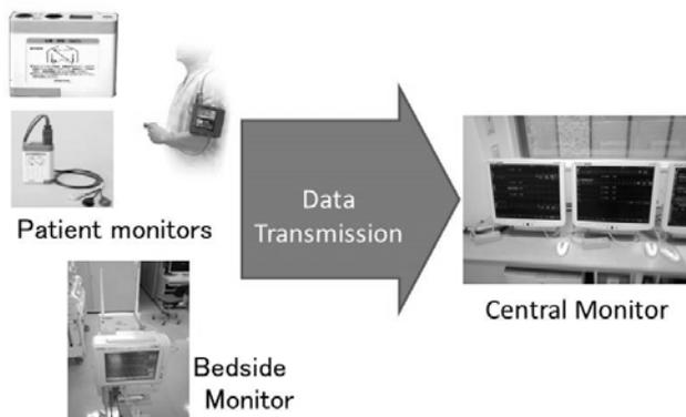
Fig.1. Medical Telemetry System
