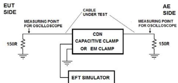
Fig.5. Measuring setup for different types of coupling networks
