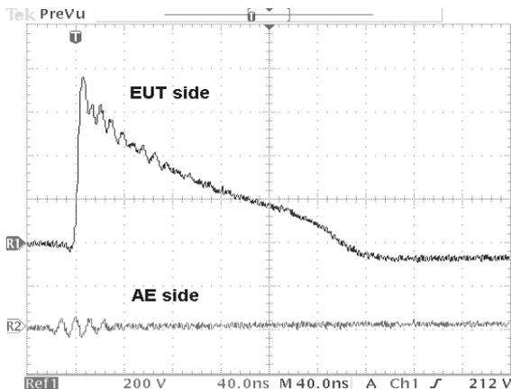
Fig.7. Output voltage of internal CDN of EFT simulator
