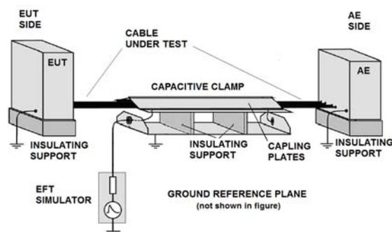
Fig.2. Test workplace arrangement with capacitive clamp
