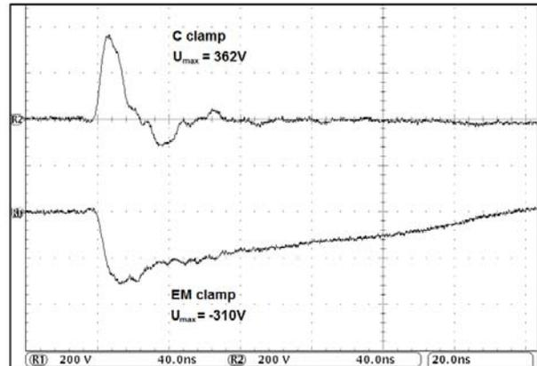
Fig.9. Output voltage of capacitive clamp and EM clamp at the AE side of CDN
