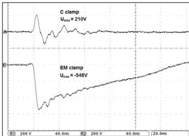
Fig.11. Output voltage of capacitive clamp and EM clamp at the AE side with overvoltage protection at the EUT side
