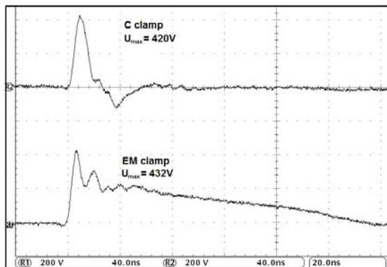
Fig.8. Output voltage of capacitive clamp and EM clamp at the EUT side of CDN
