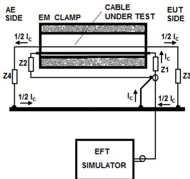
Fig.3. Simplified equivalent circuit of the capacitive coupling [4]
