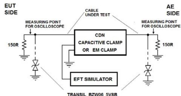
Fig.6. Measuring setup for different types of coupling networks with overvoltage protection
