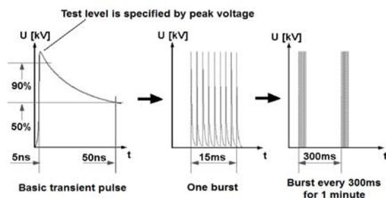
Fig.1. Standard EFT test waveform
