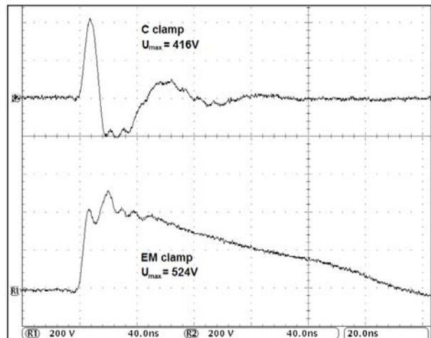
Fig.10. Output voltage of capacitive clamp and EM clamp at EUT side with overvoltage protection at AE side
