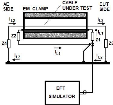
Fig.4. Simplified equivalent circuit of the inductive coupling [4]
