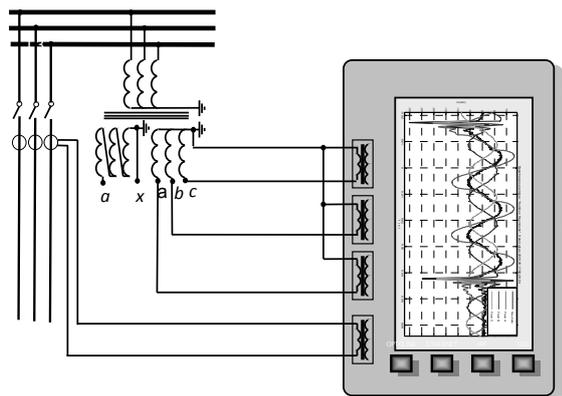
Fig 4. Scheme of connection of recorder
