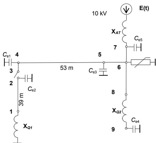
Fig. 3. Computational diagram of reactor connection
