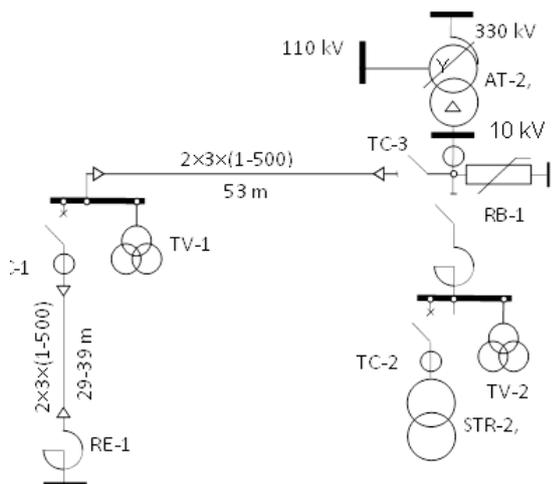
Fig. 2. Connection diagram of reactor
