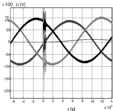
Fig. 5. Transient process of switching on of the reactor
