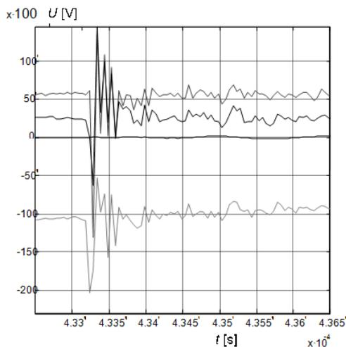
Fig. 6. Beginning of transient process of switching on of the reactor
