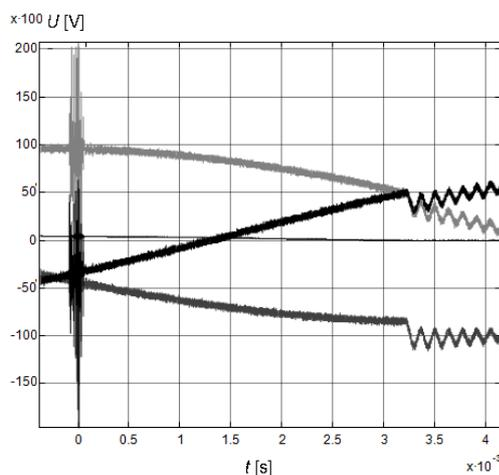
Fig. 8. Transient process of switching off of the reactor
