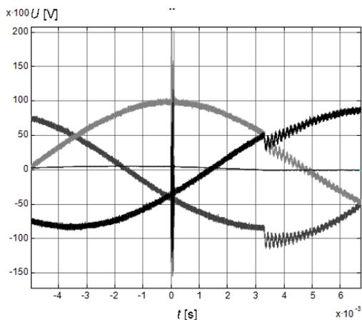
Fig. 9. Other process of switching off of the reactor
