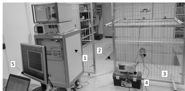
Fig.7. The antenna calibration setup: 1 – modular impulse generator, 2 – flat 4 m<sup>2</sup> metal plate, 3 – ELF-MF antenna, 4 – oscilloscope, 5 – system control.
