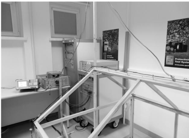
Fig.5. The measurement system. a) injection conductor connected from the bottom: 1 – horizontal conductor, 2 – down conductor, 3 – power resistor, 4 – metal ground plane connected to PE terminal, 5 – impulse current leading conductor, TG – surge generator MIG0618SS, IT – injection transformer, CP – current probe. b) injection conductor connected from the top.
