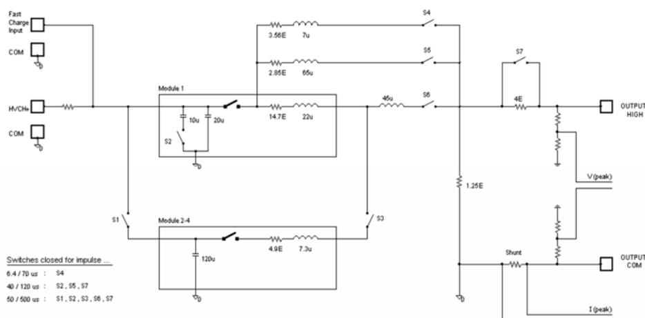
Fig.1. Simplified block diagram of high voltage part of MIG0600MS generator [5].
