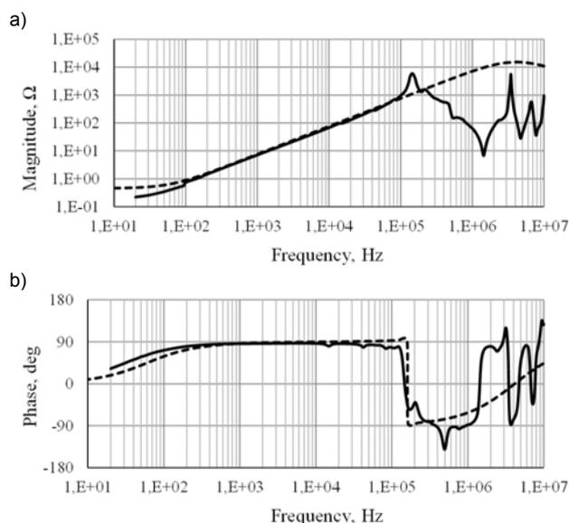
Fig.4. Frequency characteristics of input impedance of supplying transformer, measured with LCR meter (solid line) and surge generator (dashed line) between phase terminals of LV side, HV terminals were shorted: magnitude value (a) and phase (b) of LV windings.
