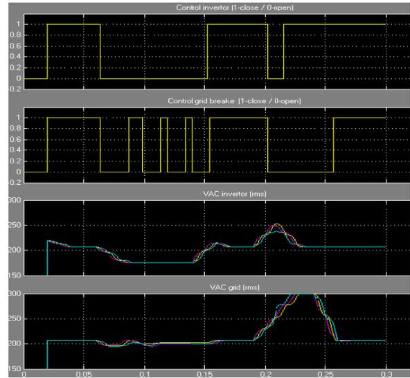
Fig. 7. Simulations for protection over/under voltage topology
