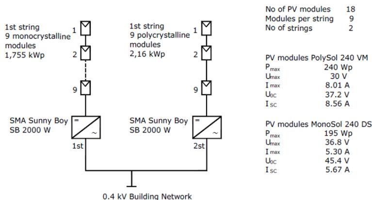
Fig.2. Schematic block circuit diagram of the PV system [12]
