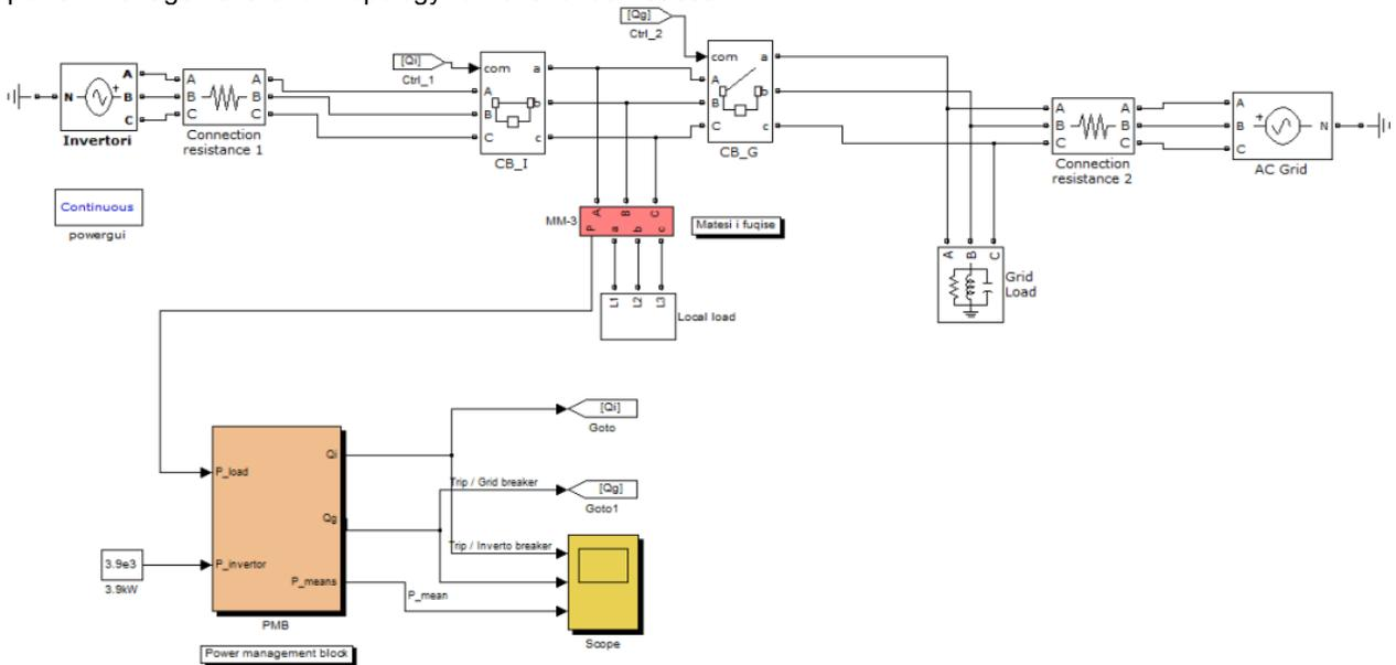
Fig. 4. Topology of the Active Power Utilization Circuit
