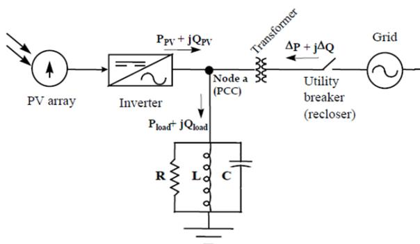
Fig.1. PV system/utility feeder configuration showing power flows [10]
