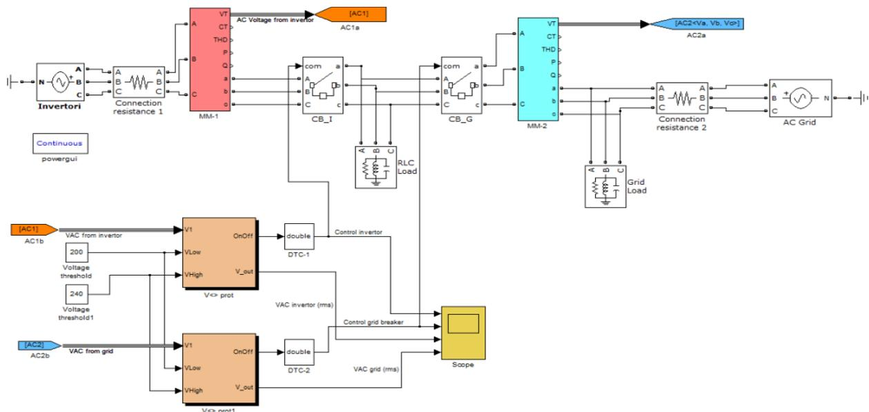
Fig. 6. Model used to simulate the method
