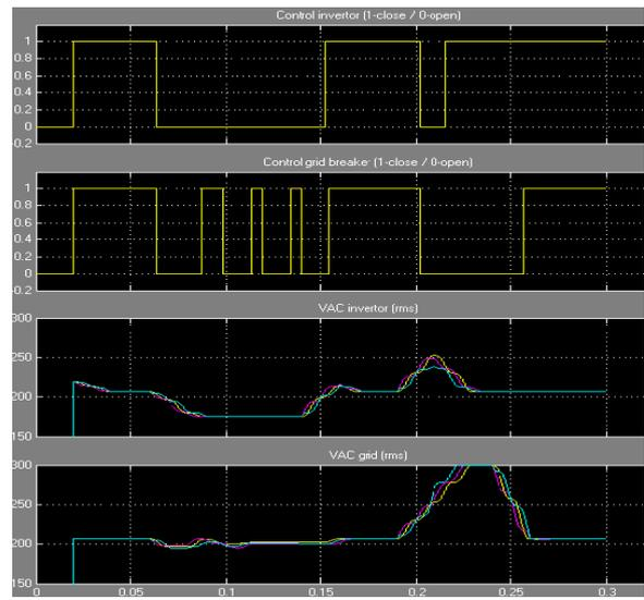
Fig. 7. Simulations for protection over/under voltage topology
