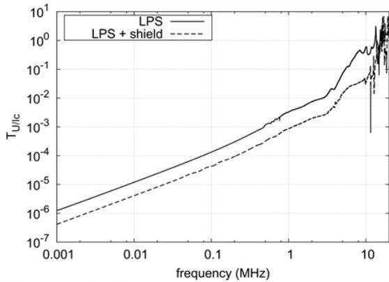
Fig. 3. Open-circuit voltage induced on the loop normalized to the current at the lightning channel base ( $T_{U/lic}$  transmittance).
