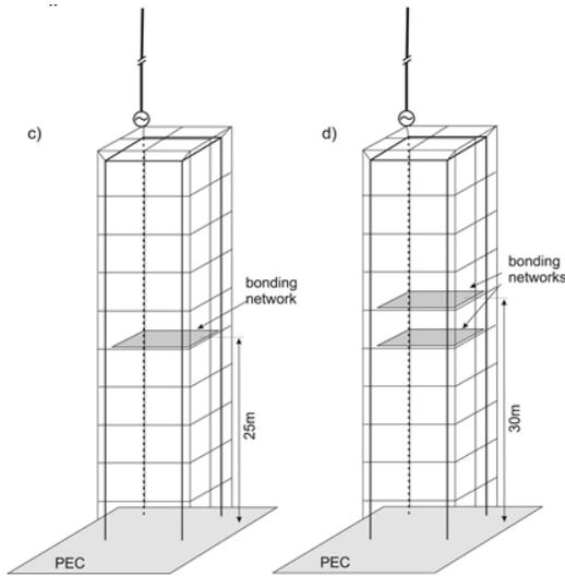
Fig. 4. Model of external LPS integrated with internal wire-grid shield with bonding networks.
