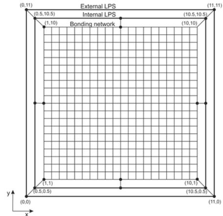
Fig. 5. Detailed structure of bonding network.
