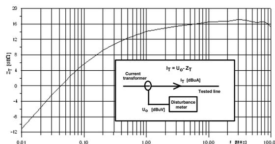
Fig. 4. Transfer impedance of current probes used to measure the disturbance current
