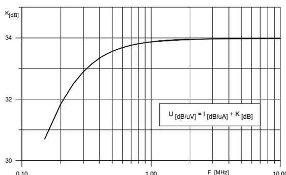
Fig. 3. Coefficient K of current probe used to measure the common disturbance voltage
