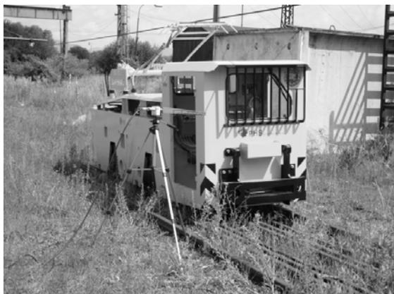
Fig. 5. Example of the device under test during RF field immunity tests
