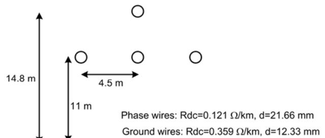
Fig.1. Three-phase overhead line under study
