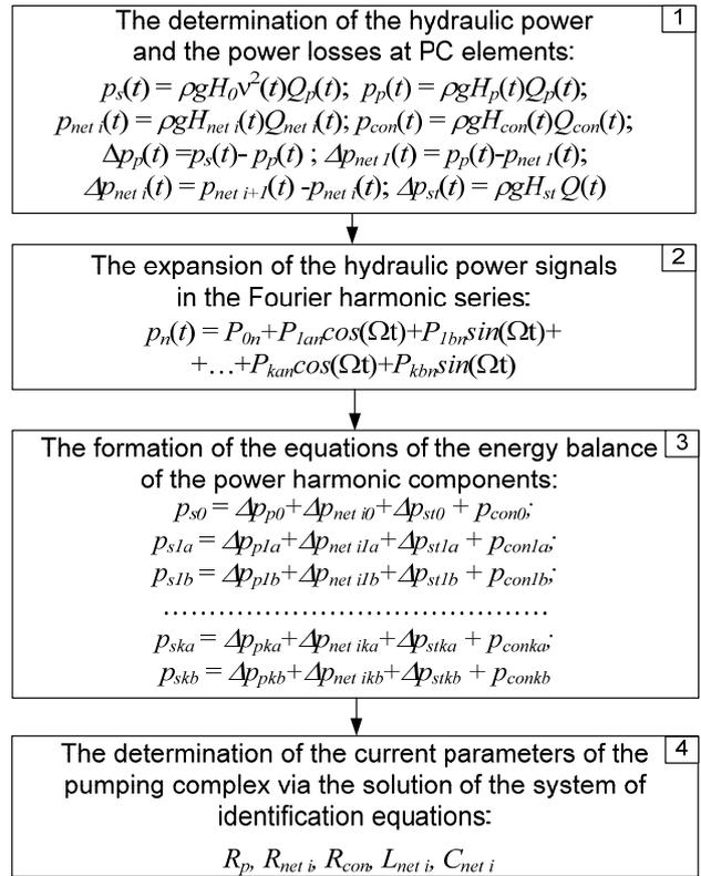
Fig. 2. The stages of the identification of PC parameters
