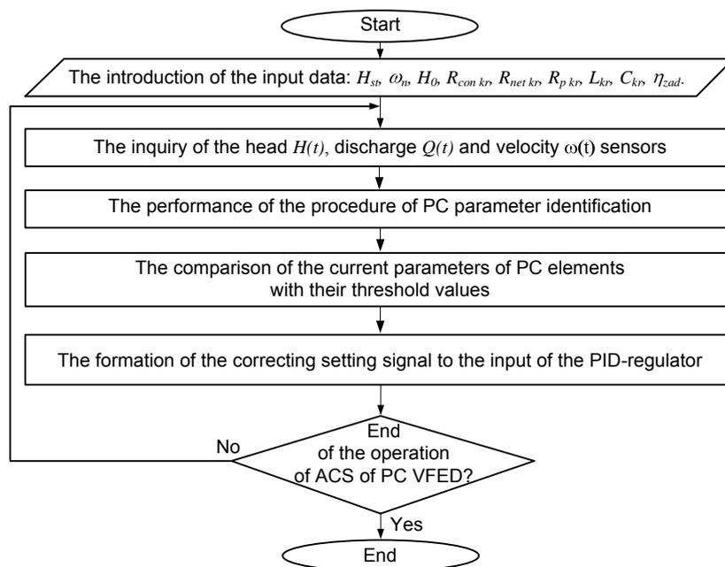
Fig. 3. The generalized algorithm of the operation of the extreme ACS of PC VFED
