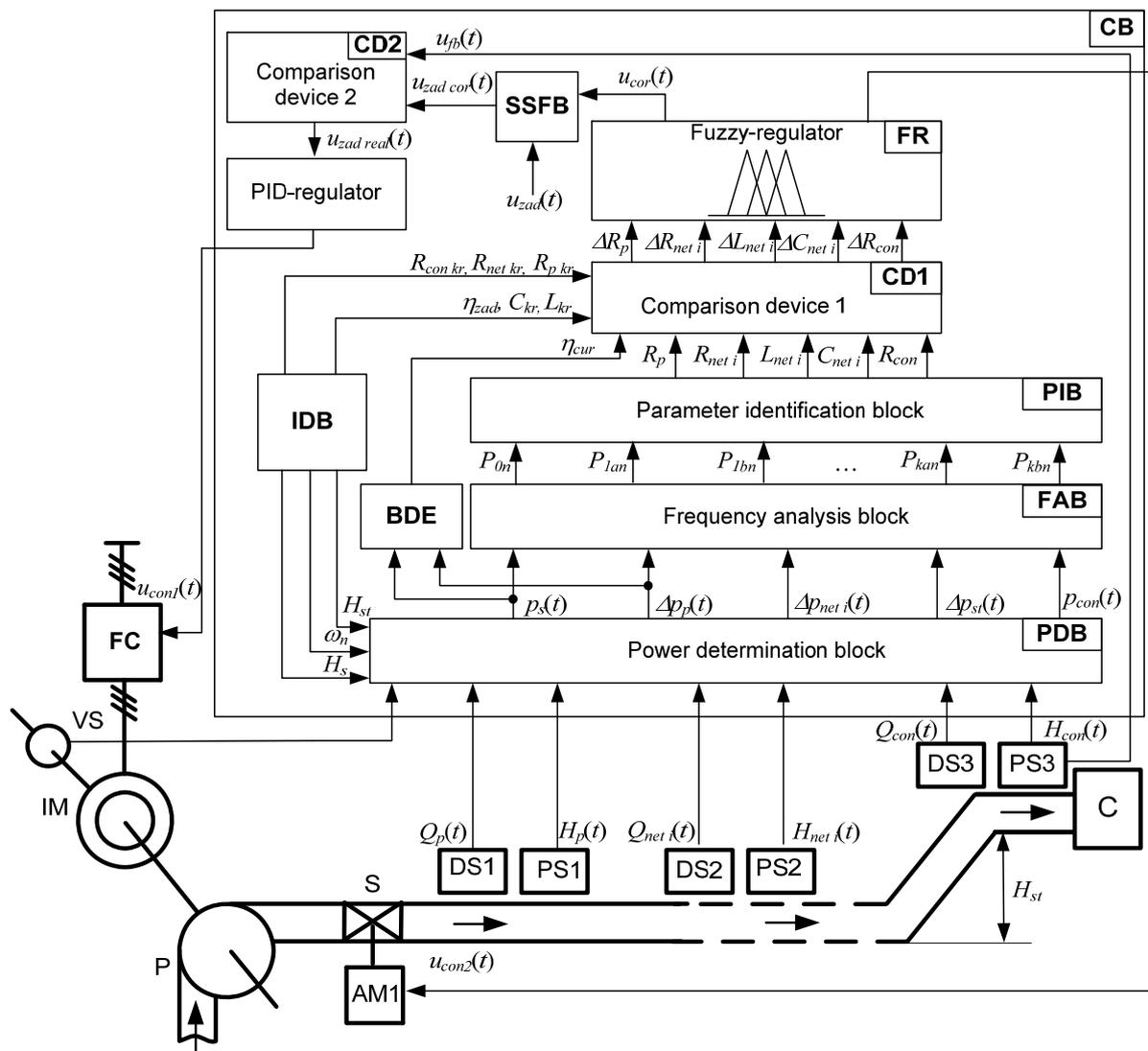
Fig. 1. A block diagram of ACS of PC VFED
