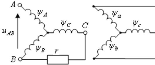
Fig.1. Computational electrical circuit of IM with an additional resistance connected in one of the phases
