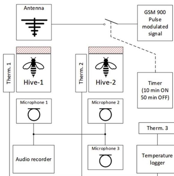
Fig. 1. Measurement setup block diagram
