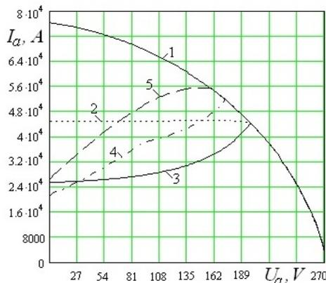
Fig. 5. External characteristics  $I_a(U_a)$  of EAF
