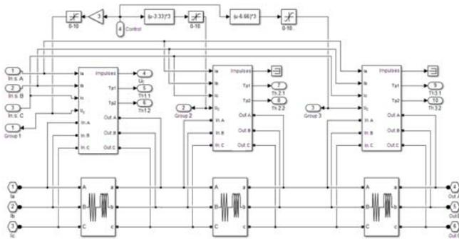
Fig. 3. Simulink-model of magneto-thyristor voltage regulator with three parallel thyristor-reactor groups
