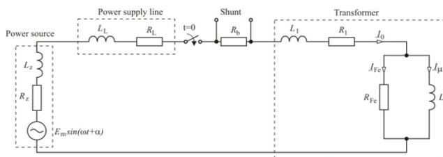
Fig. 3. Electrical circuit for measurement of the inrush current
