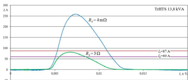
Fig. 4. Comparison of the first impulses of the inrush current when increasing the resistance of the supply network by 4 mΩ and 3 Ω
