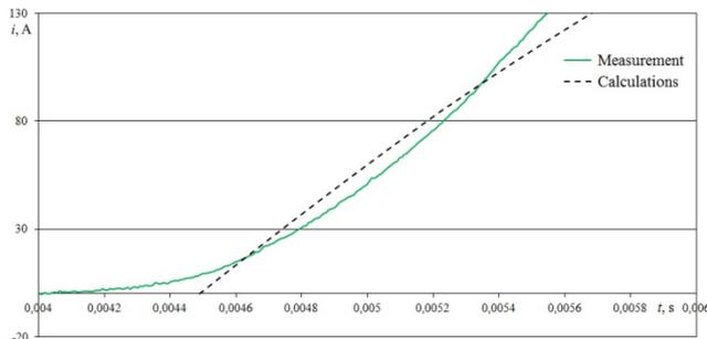
Fig. 7. Comparison of the courses of curves describing the rising edge of the first impulse of the inrush current
