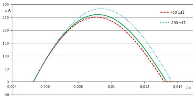
Fig. 10. Comparison of the first impulse of the inrush current at the change of the resistance of the line by +50 mΩ and -100mΩ
