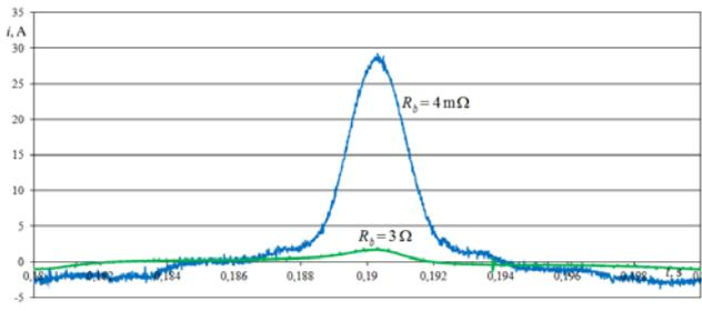
Fig. 5. Comparison of inrush currents impulses in the interval of  $0.18 \pm 0.2$  ms
