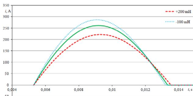
Fig. 11. Comparison of the first impulse of the inrush current at the change of the line inductance by +200 mH and -100mH
