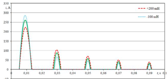
Fig. 9. Comparison of the inrush current course at the change of inductance of the line by +200 mH and -100 mH
