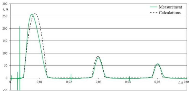
Fig. 6. Comparison of the first three impulses of the inrush currents obtained in measurements and calculations
