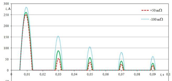
Fig. 8. Comparison of the inrush current course at the change of resistance of the power supply line by +50 mΩ and -100 mΩ
