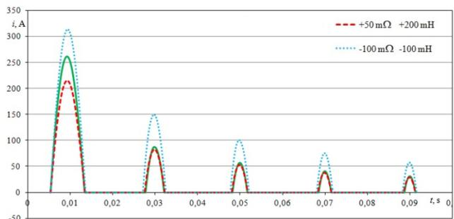
Fig. 12. Comparison of the inrush current course when the line resistance changes by +50 mΩ and inductance by +200 mH, as well as -100mΩ and -100mH
