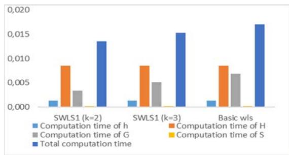
Fig.10. Computation time details in seconds for SWLS1 algorithm applied to IEEE30 bus system
