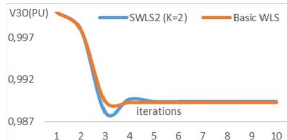
Fig.3. Evolution of estimated voltage magnitude of bus30 V30 per iteration (IEEE 30 bus system)
