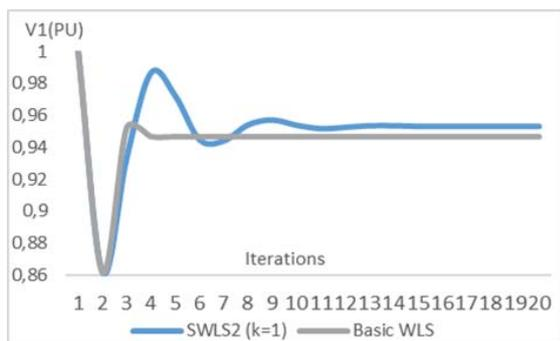
Fig.5. Evolution of estimated voltage magnitude of bus1 V1 per iteration (IEEE 118 bus system)
