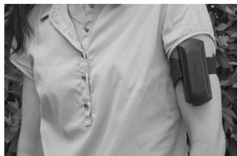
Fig. 2. An image of one of the ESM 140 dosimeters used in the tests together with the method of its installation
