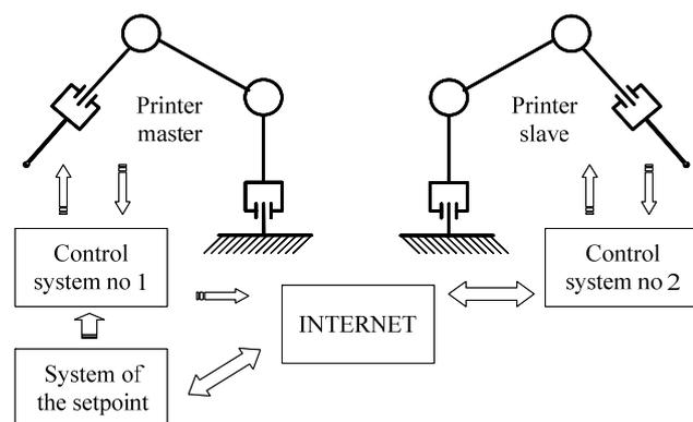
Fig. 1 Block diagram of the system of cooperating via the Internet, 3D printers
