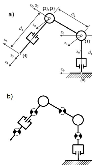
Fig.2. The described kinematic chain of robotic 3D printer - a), the position of the center of gravity members - b)
