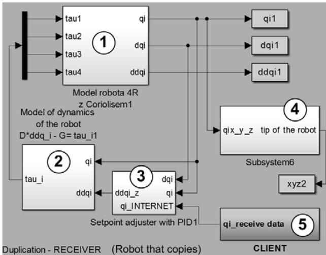
Fig.4. The implemented mathematical model of the dynamics of the manipulator 3D printer as well as its control system, working as a copier
