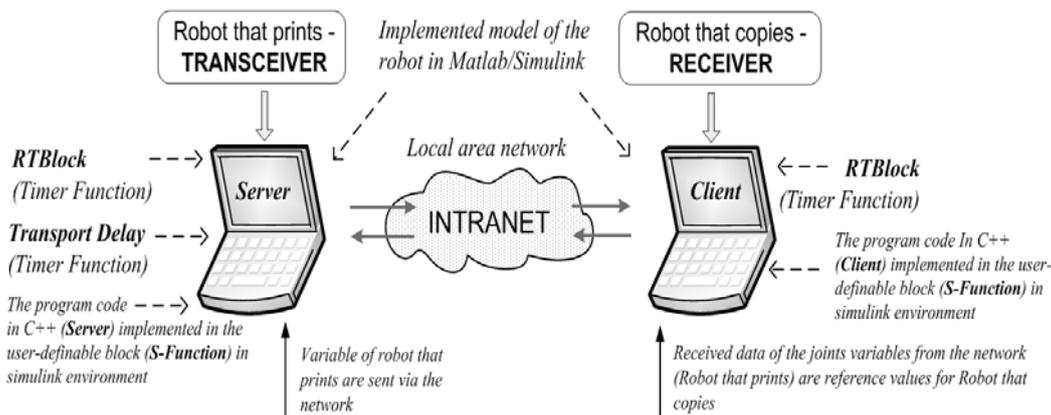
Fig. 5. Block diagram of test stand for system of cooperating 3D printers via the Intranet
