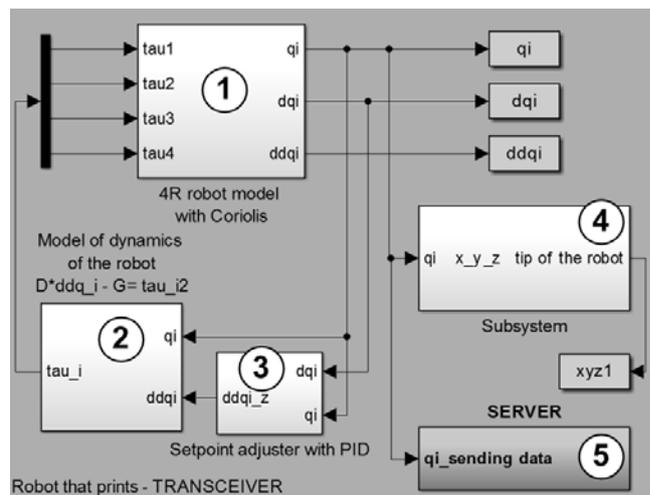
Fig.3. The implemented mathematical model of the dynamics of the manipulator 3D printer as well as its control system
