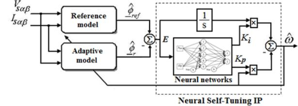
Fig.4.Structure of MRAS-Neural Self-Tuning IP observer
