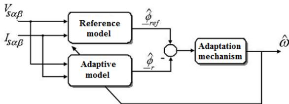
Fig.2.Structure of model reference adaptive systems
