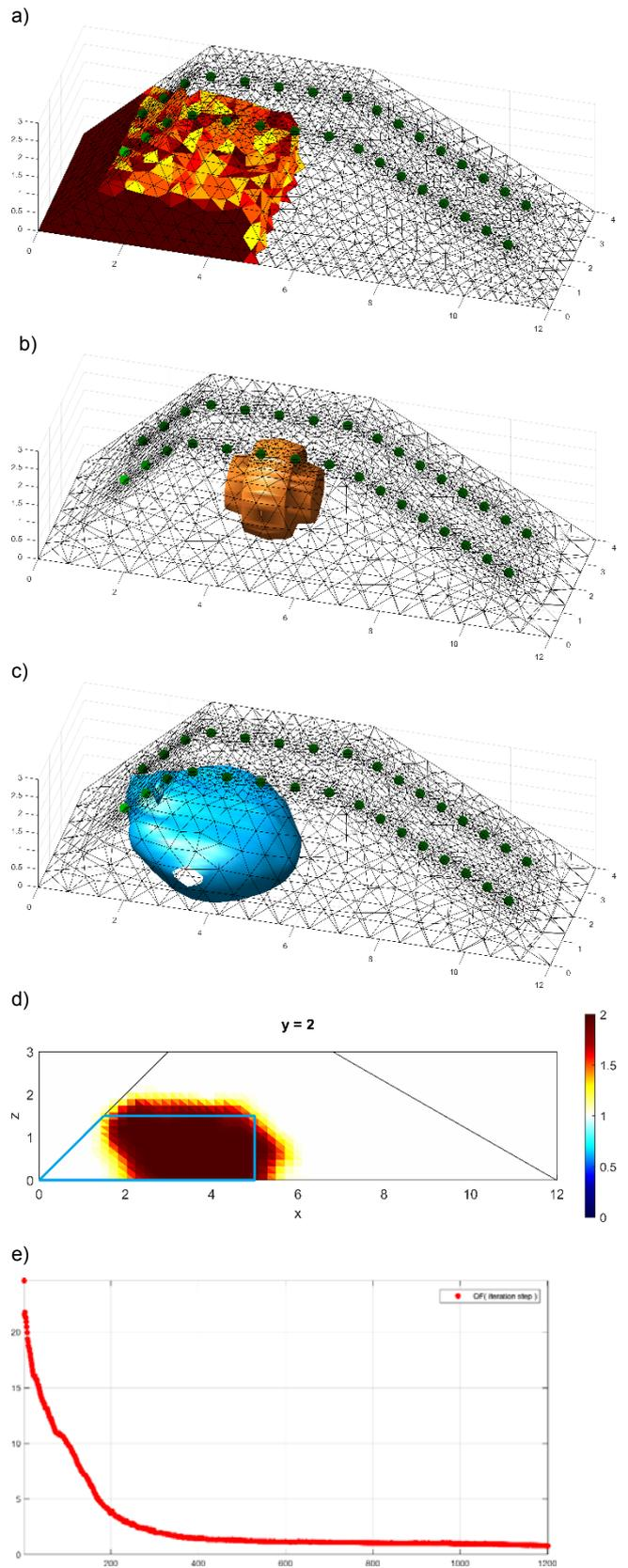
Fig. 5. Image reconstruction by the level set method: a) model, b) zero-level set, c) final level set, d) conductivity on the cross-section - plane  $\{y - 2.0 = 0\}$ , e) objective function in the next iterative steps.
