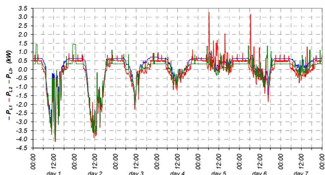
Fig. 5. Active powers  $P_{L1}$ ,  $P_{L2}$ ,  $P_{L3}$  at the connection node of the PV system
