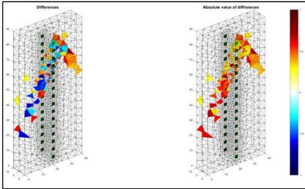
Fig. 6. The damp cellular concrete block and reconstruction based on the Least Angle Regression with 2 side measurements (2x16 electrodes) – model III.
