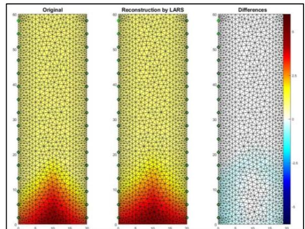
Fig. 3. The damp cellular concrete block and reconstruction based on the Least Angle Regression with 2 side measurements – model, reconstruction and differences.
