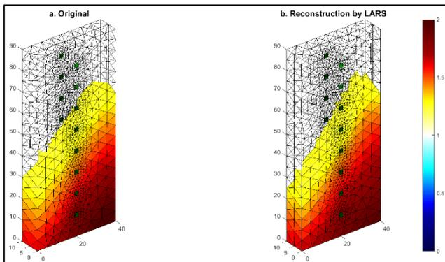
Fig. 4. The damp cellular concrete block and reconstruction based on the Least Angle Regression with 2 side measurements (2x8 electrodes) – models of moisture I.
