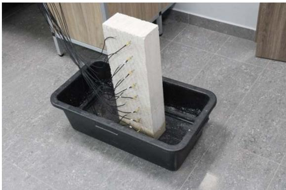
Fig. 1. Measurement systems - the laboratory airbrick model.
