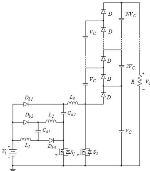
Fig. 5. N-level dual charge-pump DC-DC converter
