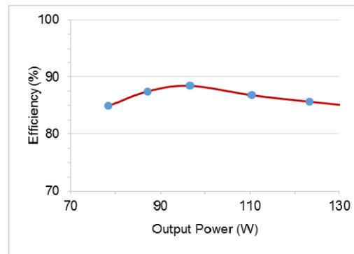
Fig. 9. Efficiency against output power of the proposed converter
