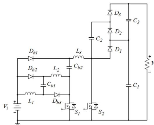
Fig. 1. Proposed dual charge-pump multilevel converter
