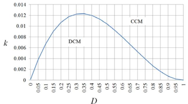
Fig. 4. Boundary condition between CCM and DCM
