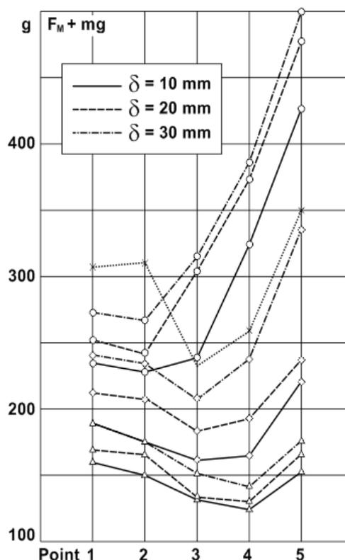
Fig. 3. Experimental curves representing the distribution of the force field across the width of the suspended iron separator working zone at the depth of extraction
