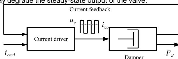
Fig. 1. MR damper system,  $i_{cmt}$  – current command,  $i_{co}$  – coil current,  $u_c$  – supply voltage,  $F_d$  – force [5]
