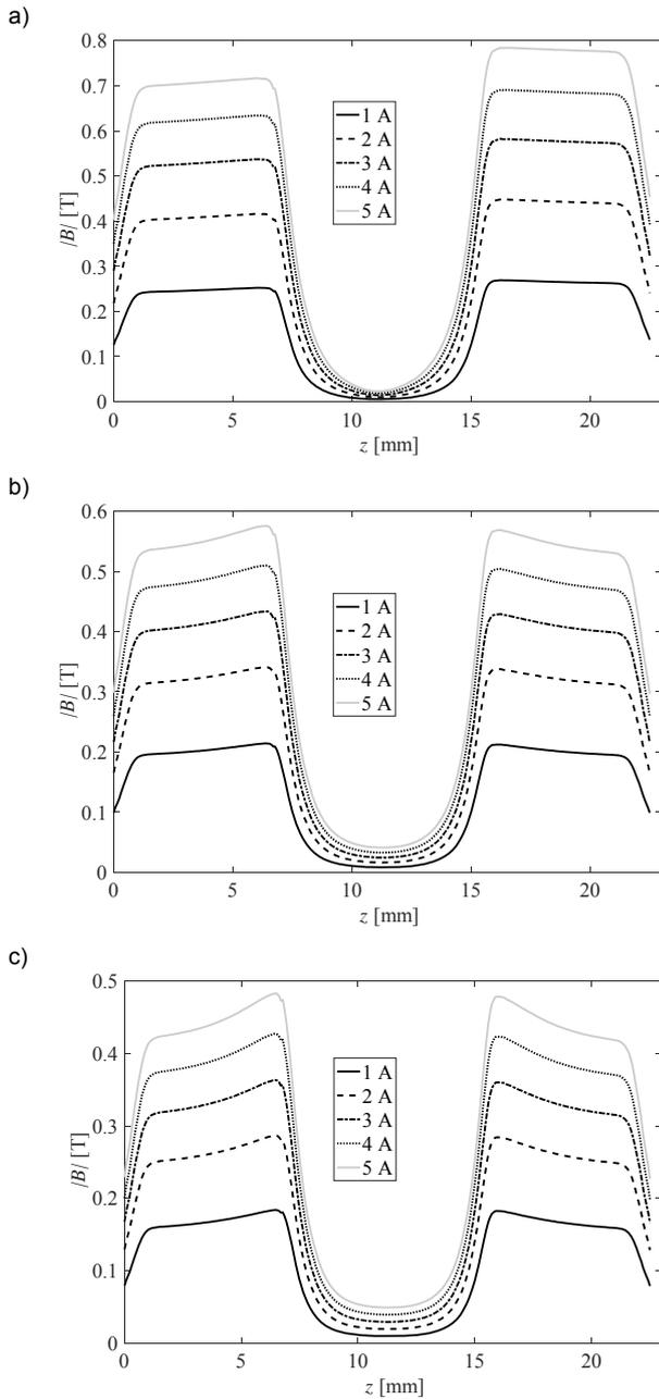
Fig. 10. Flux density vs. current in the flow channel at various frequencies: a)  $f=5$  Hz, b)  $f=25$  Hz, c)  $f=50$  Hz.
