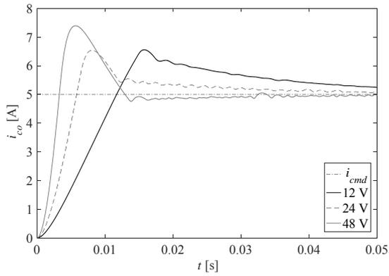
Fig. 14. Supply voltage impact ( $I_{cmd}=5$  A,  $K_p=10$ ,  $K_i=50$ , anti-windup: off)
