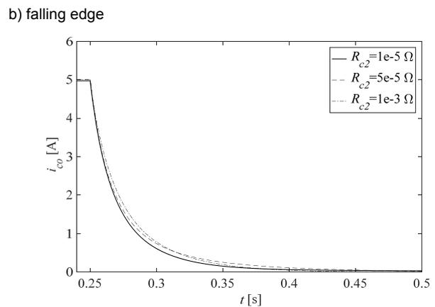
Fig. 18. Parasitic resistance impact: unregulated response ( $k_c=0.4$ )
