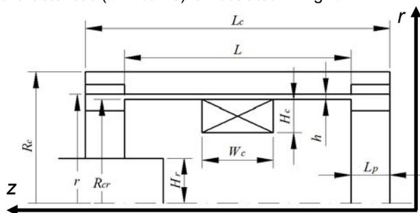
Fig.2. Geometry of a single coil MR valve assembly
