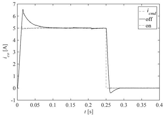
Fig. 16. PID component setting: anti-windup on/off ( $I_{cmd}=5$  A)
