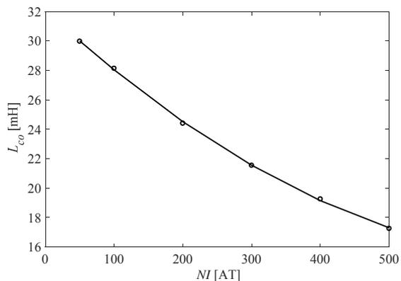
Fig. 8. Coil inductance vs. coil ampere turns
