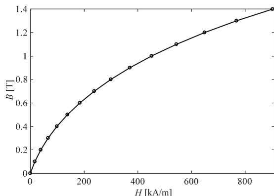
Fig.3. Magnetisation characteristics of the MR fluid [3],  $B$  – flux density,  $H$  – magnetic field strength
