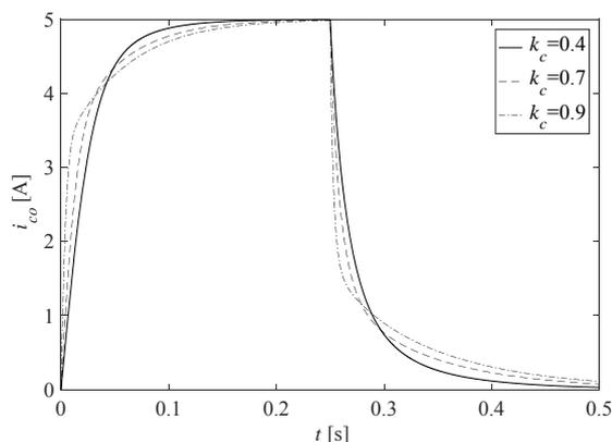
Fig. 19. Coil coupling factor: unregulated response ( $R_2=50 \mu\Omega$ )
