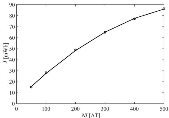
Fig. 7. Computed flux linkage vs. coil ampere turns
