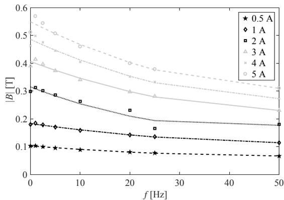
Fig. 11. Averaged flux density  $|B|$  vs frequency  $f$  and current  $I_{co}$ .
