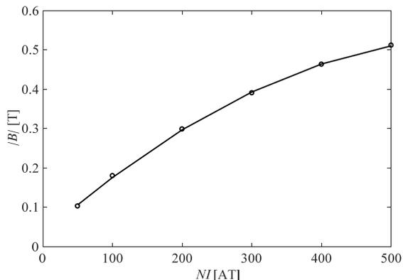
Fig. 6. Averaged flux density vs. coil ampere turns
