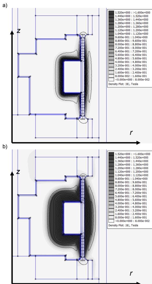
Fig. 9. Flux density distribution at  $f=50$  Hz at: a) 100 AT turns, b) 500 AT
