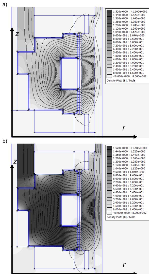
Fig.4. Flux density  $|B|$  distribution and flux lines: a) 100 AT, b) 500 AT
