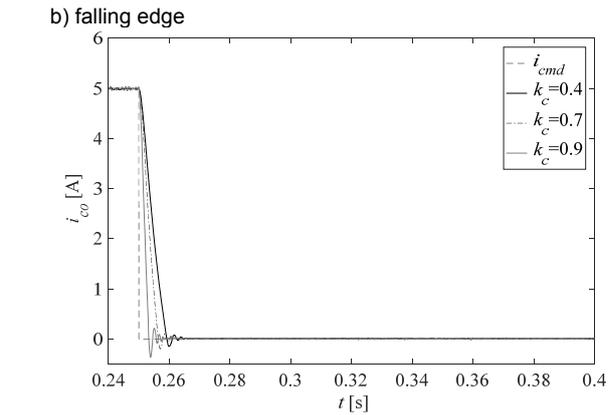
Fig. 17. Impact of the coupling factor  $k$  (anti-windup: on)
