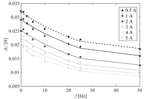
Fig. 13. Coil inductance vs. frequency and current
