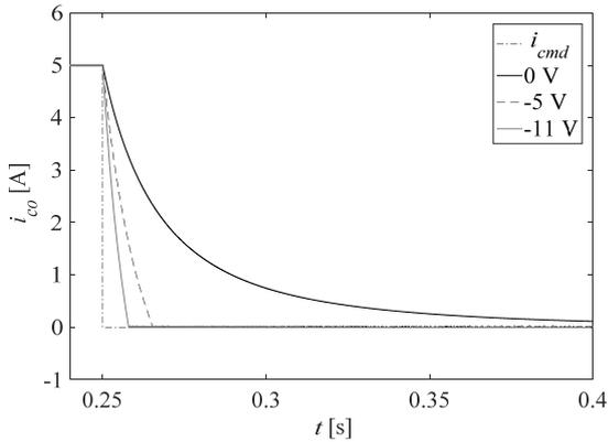
Fig. 15. Turn-off voltage impact ( $I_{cmd}=5$  A,  $K_p=10$ ,  $K_i=50$ , anti-windup: off)
