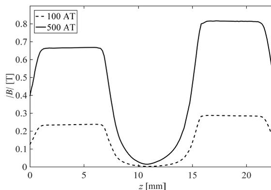
Fig.5. Computed flux density variation in the flow channel
