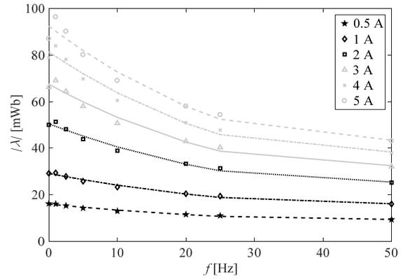
Fig. 12. Flux linkage vs. frequency and current
