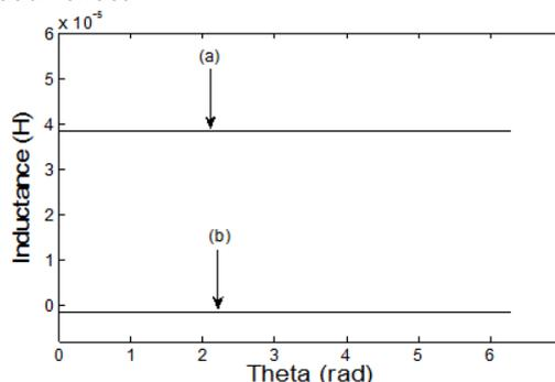
Fig.5. Magnetizing and mutual rotor inductance without saturation 'a' and 'b' (a) magnetizing, (b) mutual
