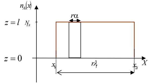
Fig.2. Distribution function of a stator coil.  $A_i$ .
