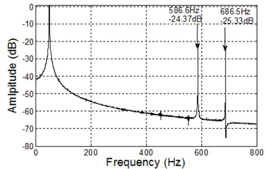
Fig.10. Spectrum of the stator current for the case of a healthy motor operation without taking into account the saturation effect.
