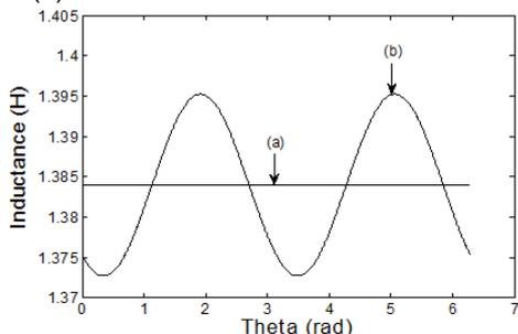
Fig.3. Magnetization inductance as a function of the position of the stator. (a) without saturation, (b) with saturation
