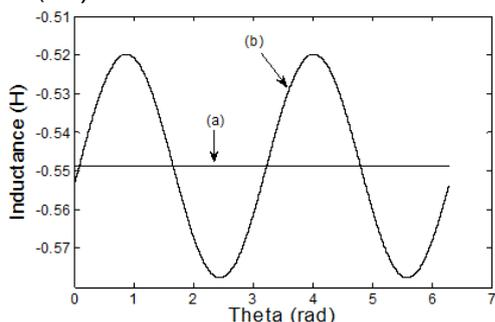
Fig.4. Mutual inductance between the stator phases 'a' and 'b' (a) without saturation, (b) with saturation.
