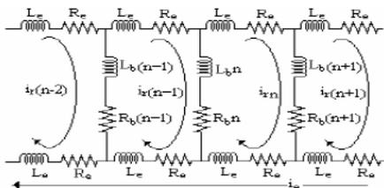
Fig.1. Mesh circuit of the cage rotor
