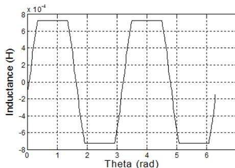
Fig.6. Mutual inductance between the first stator phases 'a' and the first rotor cell without saturation.
