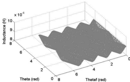
Fig.8. Magnetizing inductance of the first rotor mesh with saturation
