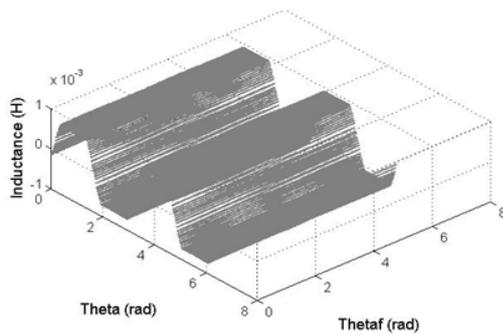
Fig.7. Mutual inductance between the first stator phases 'a' and the first rotor mesh with saturation
