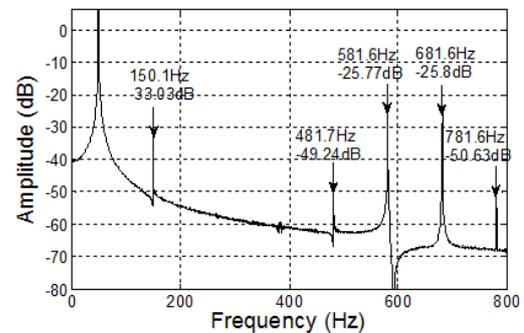
Fig.11. Spectrum of the stator current for the case of an operation without and with the saturation effect.
