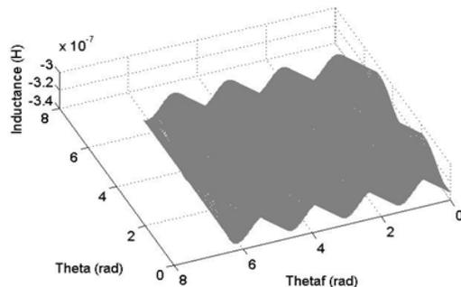
Fig.9. Mutual inductance between the first rotor mesh and the second rotor mesh with saturation.
