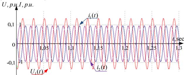
Fig. 9. Oscillograms of the current, voltage of primary winding and the current of secondary winding of  $\xi$ -phase of the SPT in short-circuit test
