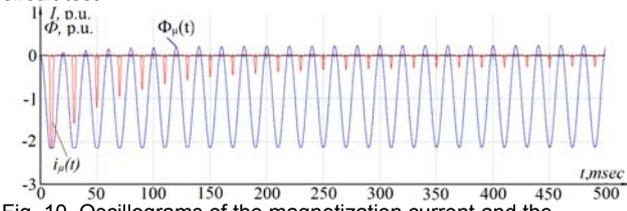
Fig. 10. Oscillograms of the magnetization current and the magnetic flux of  $\xi$ -phase of the SPT in on-load test
