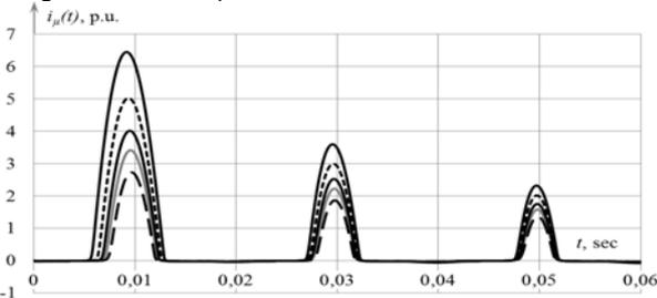
Fig. 8. Oscillograms of the magnetization current of SPT at various parameters in open-circuit test
