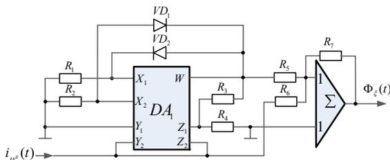
Fig. 3. Functional converter for continuous simulation of the magnetization curve
