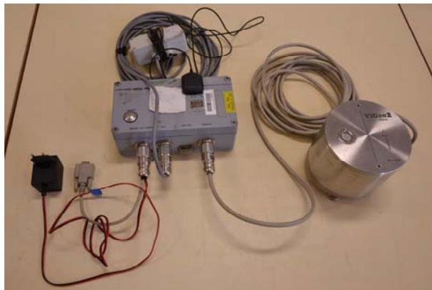
Fig.1. Seismic apparatus Gaia2T with seismometer ViGeo2
