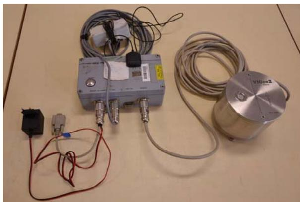
Fig.1. Seismic apparatus Gaia2T with seismometer ViGeo2
