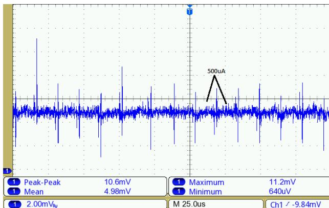
Fig.8. Current consumption profile for MSP432P401R normal run
