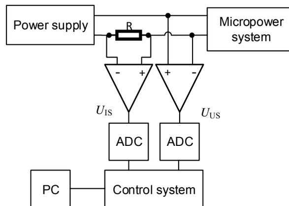
Fig. 1. Energy measurement method implementation using energy definition
