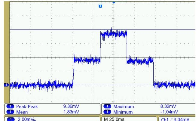
Fig.5. Current consupption profile for BME280 sensor
