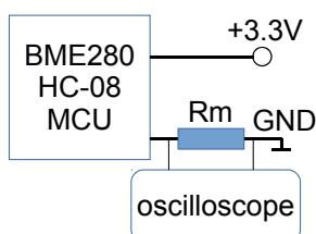
Fig.4. Measurement setup for current consumption profile acquisition
