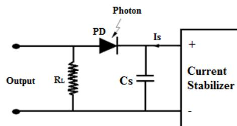
Fig. 1. Constant current temperature compensation.
