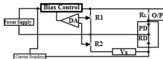
Fig.2. Constant current power supply for Photodiode (PD).
