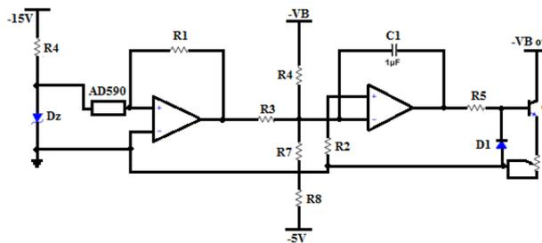
Fig.3. Circuit schematic for temperature compensation.
