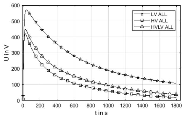
Fig .5. RV-curves measurements on TR3 ( $U_p = 1$  kV,  $t_p = 1800$  s)
