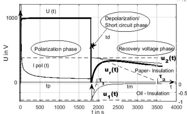
Fig. 1. Basic principle of the measurements according to PCRVR
