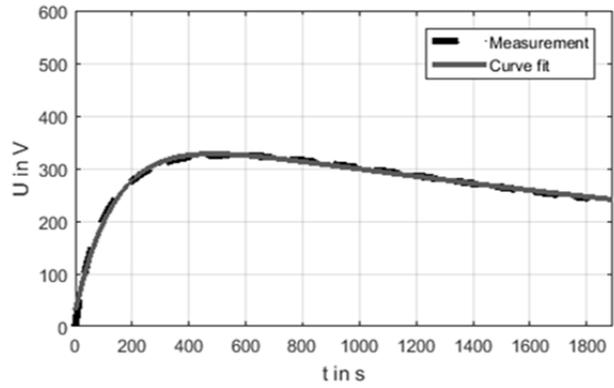
Fig.8. Curve fit for TR2 at LV ALL with 3 elements
