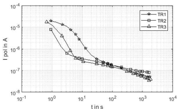
Fig.2. Polarization current  $I_p$  for 3 units at 1 kV (LV-All setup)
