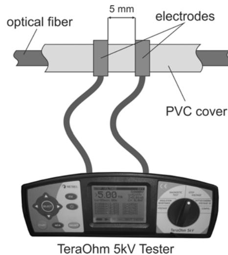
Fig. 3. A schematic view of a setup for measurements of isolation resistance of optical fibers
