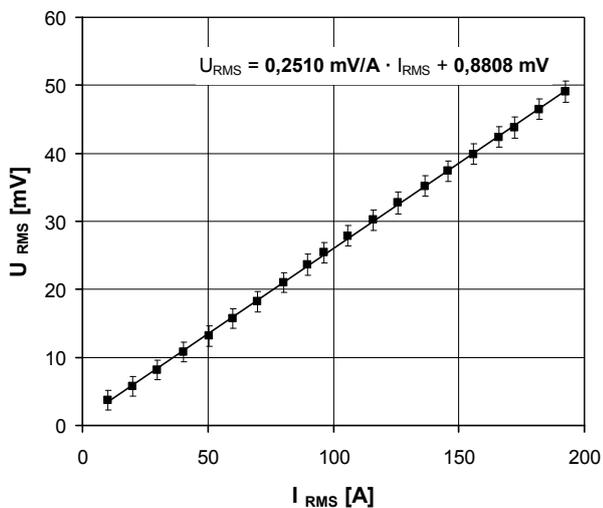
Fig.5. The response of the sensor as a function of electric current intensity in busbar for voltage 0 kV
