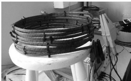
Fig.3. 8-turns air coil model
