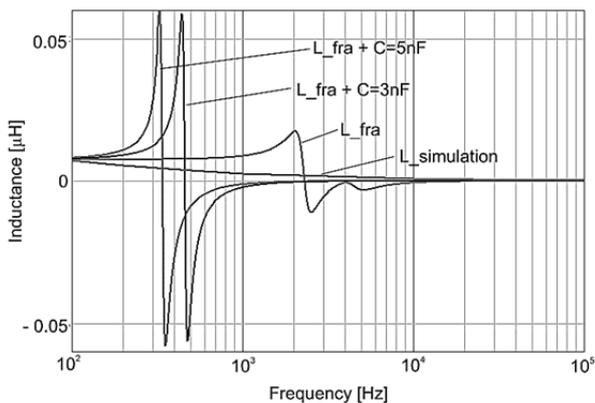
Fig.9. The influence of additional capacitances on occurrence of resonance in FRA measurements
