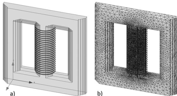
Fig.5. 24-turns coil model in FEM software, a) computation domain (1/2 of the model due to symmetry of the object), b) finite element mesh
