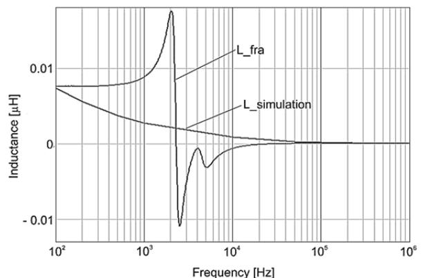
Fig.8. Inductance of the 24-turns coil calculated for computer model and measured on actual coil as a function of frequency
