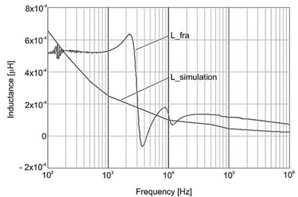
Fig.7. Inductance of the 8-turns coil calculated for computer model and measured on actual coil as a function of frequency
