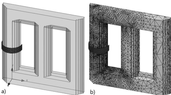
Fig.4. 8-turns coil model in FEM software, a) computation domain (1/2 of the model due to symmetry of the object), b) finite element mesh
