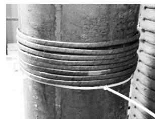
Fig.2. 8-turns coil wound with rectangular cross-section wire mounted on the pressboard tube
