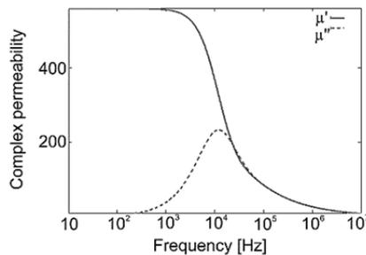
Fig.6. Complex permeability of ferromagnetic laminated material ( $\mu_r = 560$ ,  $\gamma = 10^6$  S/m,  $2D = 0,22$  mm) as a function of frequency
