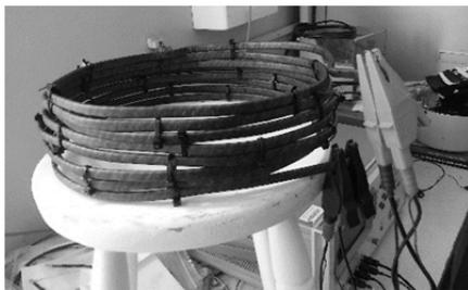
Fig.3. 8-turns air coil model
