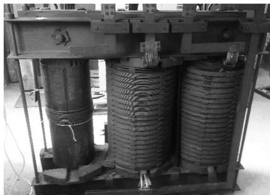
Fig.1. The coil wound on the first column of laminated, distribution transformer core and the factory windings (both LV and HV) mounted on the other two columns.
