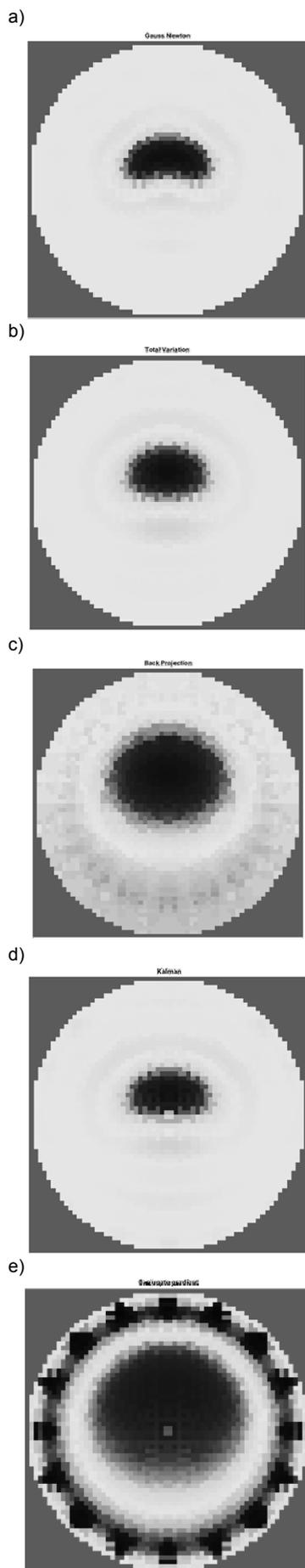
Fig. 7. Image reconstruction: a) Gauss-Newton, b) Total Variation, c) Back Projection, d) Kalman, e) Conjugate Gradient
