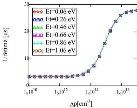
Fig.1. Dependence of the lifetime of carriers on the concentration of excess minority carriers  $\Delta p$  for different values of  $Et$
