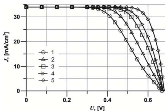
Fig.7. Simulation of dependences  $J = f(U)$  of illuminated HIT-IBC solar cell, calculated for different values of band gap  $E_g$  of the intrinsic a-Si buffer layer: 1 – 1,72 eV, 2 – 1,70 eV, 3 – 1,68 eV, 4 – 1,665 eV, 5 – 1,65 eV [12]
