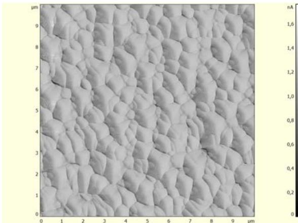
Fig.4. SEM micrograph showing the front surface of the examined HIT-IBC solar cell
