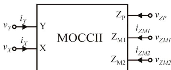
Fig.1. Graphical symbol of proposed multiple output second-generation current conveyor (MOCCII) block
