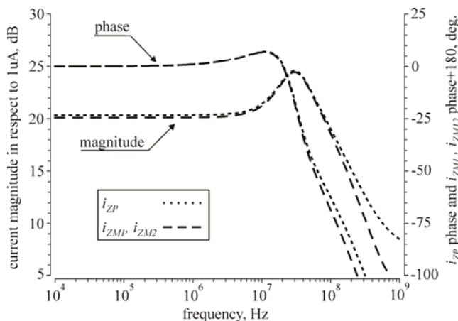
Fig.5. Simulated small signal frequency responses of the MOCCII from Fig. 3, as input voltage source feed to Y terminal was used, X terminal was connected through 100kΩ resistor to the ground, output currents were tested at shorts to the ground
