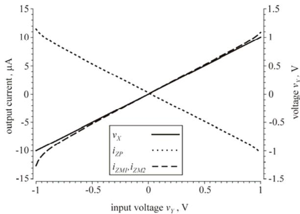
Fig.4. Simulated DC transfer characteristics of the MOCCII from Fig. 3, as input voltage source feed to Y terminal was used, X terminal was connected through 100kΩ resistor to the ground, output currents were tested at shorts to the ground
