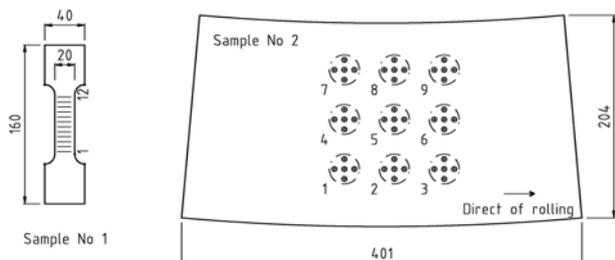
Fig.4 Dimension and measurement points localization of the investigated samples.
