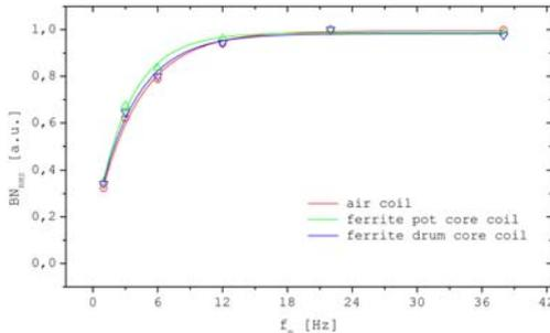
Fig.10 Variation of the normalized  $BN_{RMS}$  with magnetization frequency  $f_m$
