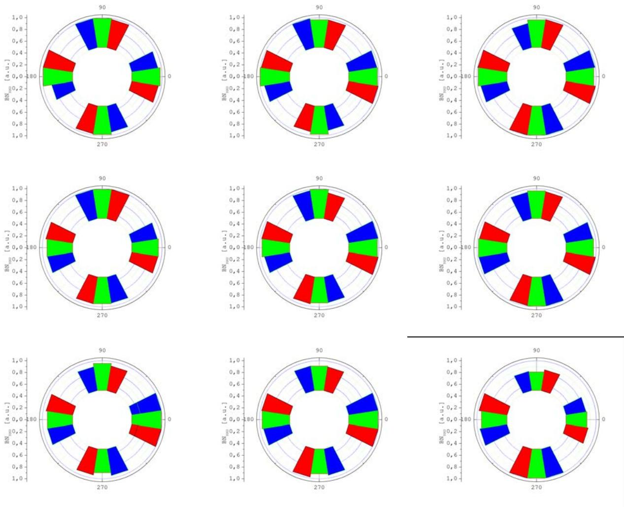
Fig. 15 Normalized values of  $BN_{RMS}$  in measurement points on the steel sheet sample; red – air coil, green - pot core coil, blue – drum core coil
