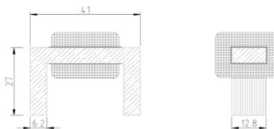
Fig.2 Schematic view of magnetization yoke used during study
