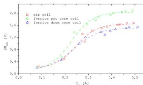
Fig.7 Variation of the  $BN_{RMS}$  with magnetization current  $I_m$
