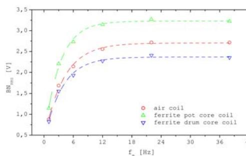
Fig.8 Variation of the  $BN_{RMS}$  with magnetization frequency  $f_m$
