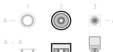
Fig.3 Schematic view of BN detection sensors used in experiments
