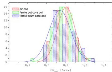
Fig.14 Categorized data of multipoint BN measurements in the steel sheet sample.
