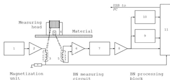
Fig.1 Block diagram of measurement set-up: 1 – saw-tooth generator, 2 – current power amplifier, 3 – magnetization coil, 4 – yoke, 5- detection coil, 6 – preamplifier, 7 – high pass filter, 8 – amplifier, 9 – RMS converter, 10 – envelope detector, 11 – DAQ unit, R – resistor (1 $\Omega$ )
