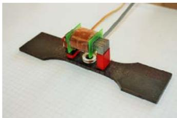
Fig.11 Details of experiment on the first sample - air coil sensor.
