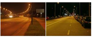
Fig.1. Geometrically structured, regular line of the points of light (optical arrangement) and high uniformity of illumination of the road determine the aesthetics of street lighting to the greatest extent.
