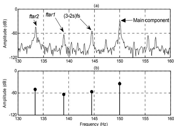
Fig. 3. Example of application of the frequency tracking module. (a) Spectrum of the zero sequence voltage (b) Result of frequency tracking module
