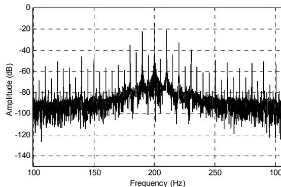
Fig. 4. Zero sequence voltage result in case of motor supplied with inverter and 2 broken rotor bars under 3/4 of load
