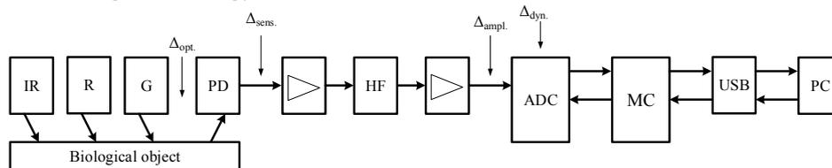
Fig. 2. Generalized structure of measuring channel of optical-electronic device for diagnosis the peripheral blood circulation
