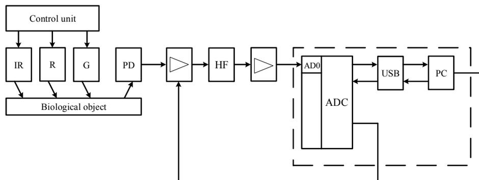
Fig.1. Block diagram of the optical-electronic photoplethysmographic multispectral device for diagnosis of the peripheral blood circulation
