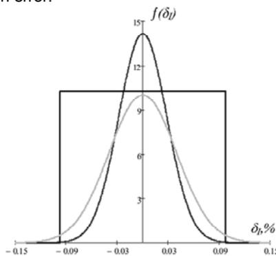
Fig.3. The composition of distribution laws of the total measurement error
