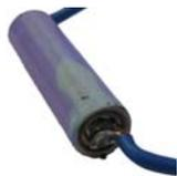
Fig.21. View of Li-Ion 2200mAh battery, after the short circuit test
