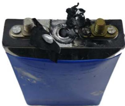
Fig.16. View of LiFePO4 8Ah battery, after the short circuit test
