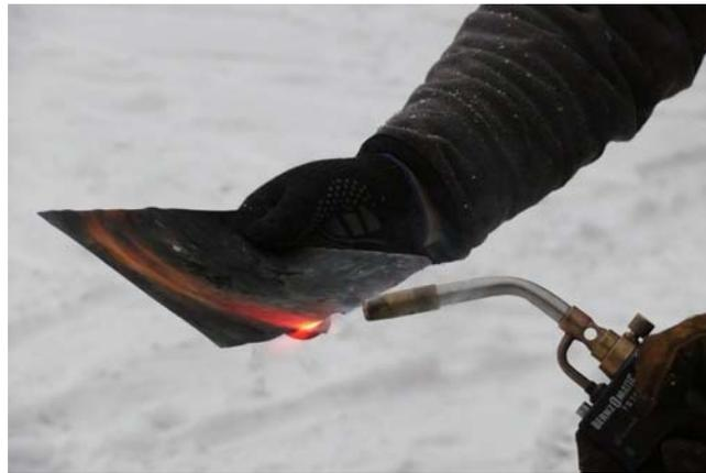
Fig.17. An unsuccessful attempt of ignition of LiFePO4 battery plate
