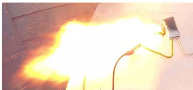
Fig.13. View of Li-PO 1000mAh battery during overcharge test at 2C which ended with explosion and fire
