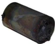
Fig.23. View of Li-SOCl<sub>2</sub> 13Ah battery, after the short circuit test
