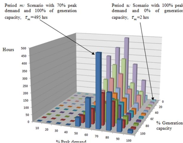
Fig.2. Coincident hours for each scenario of load and generation
