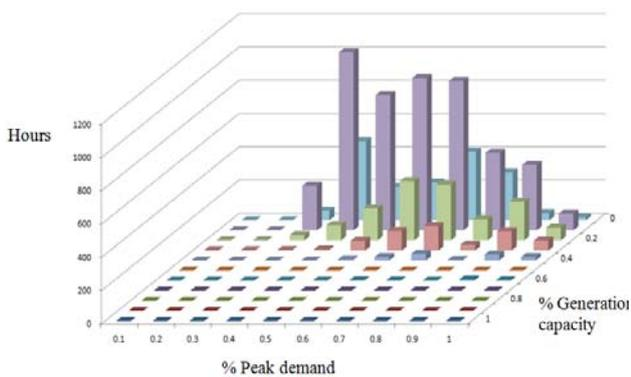
Fig.4. Coincident hours of load demand and generation in each interval.
