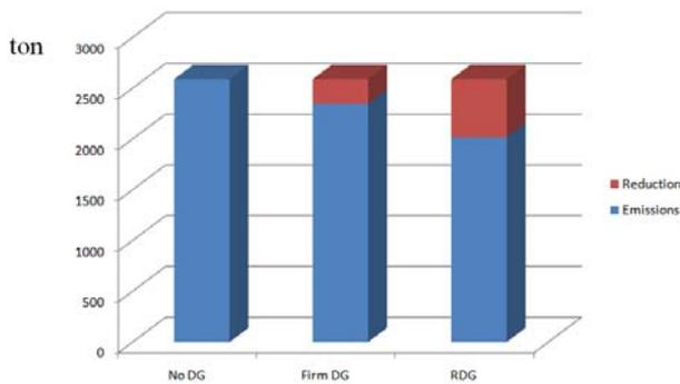
Fig.5. Total reduction of CO<sub>2</sub> emissions during the year.
