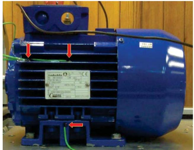
Fig. 6. Mountings of thermocouples
