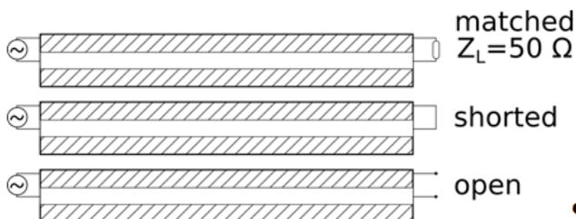
Fig. 2. Three types of termination of coaxial cable
