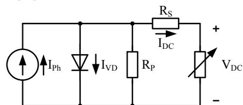
Fig.1. An equivalent electric circuit of solar battery
