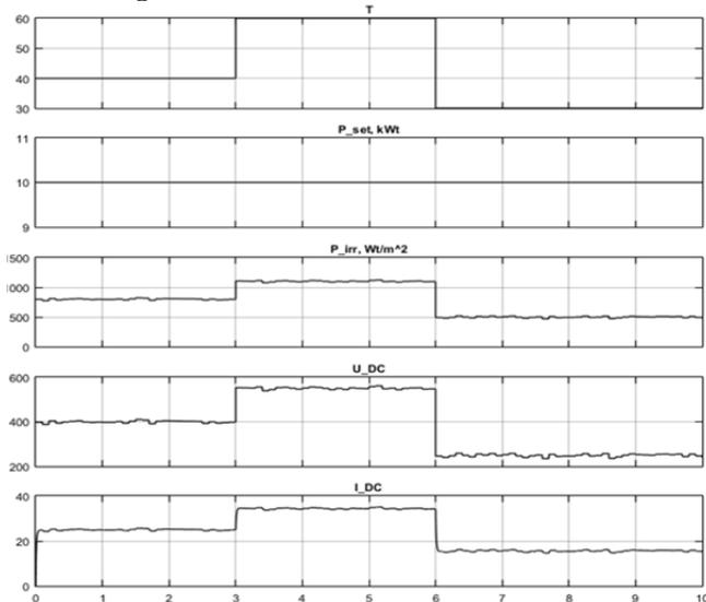
Fig.12. Temperature, the set and the actual value of light level, the output current and voltage of the solar battery
