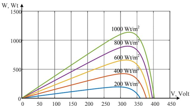
Fig.2. Graph of power relationships, which may be produced by a solar module to grid inverter during the operation with the actual output voltage
