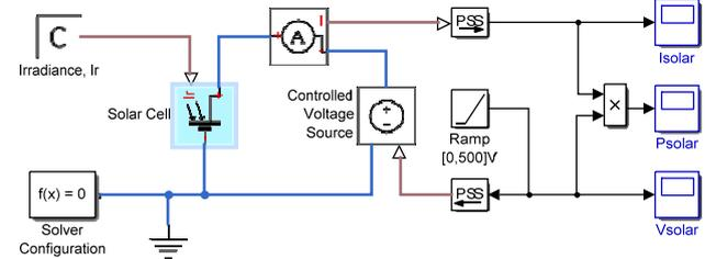
Fig.3. Block diagram of the model for solar cell power curve
