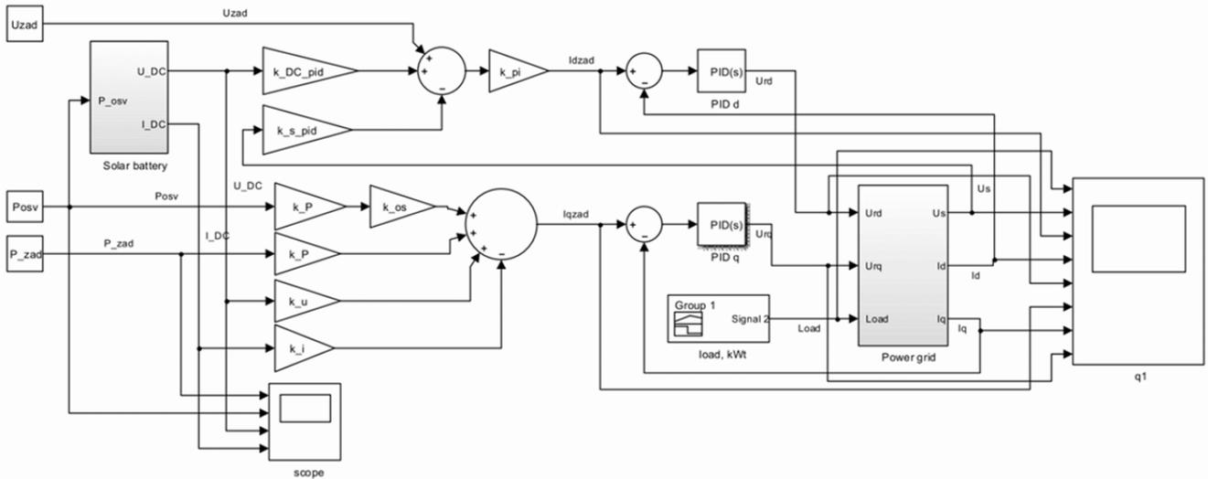
Fig.6. The computer model to test the adequacy of control of  $d$  and  $q$  current components of power inverter:  $U_{zad}$  – set grid voltage value;  $P_{osc}$  – power value that is perceived by lighting;  $P_{zad}$  – set voltage value of solar module; PID  $d$  – PID controller of the longitudinal component of the current of inverter; PID  $q$  – PID controller of the transverse component of the current of inverter; load – load preset schedule; Power grid – network model
