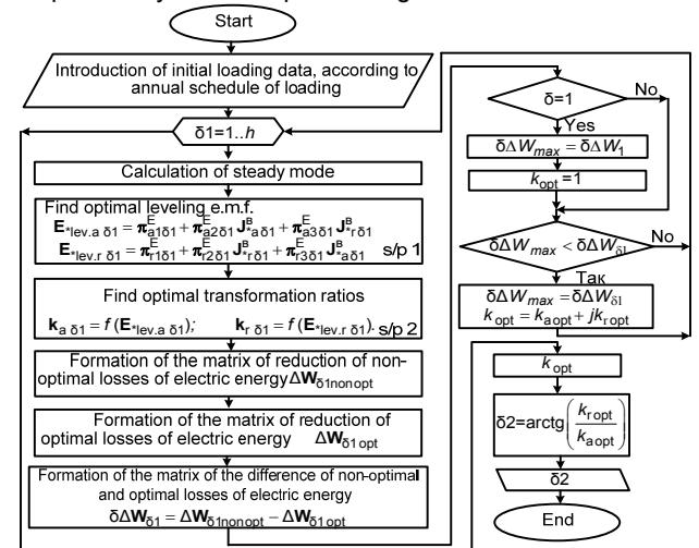
Fig.2. Block diagram of the algorithm for determining the optimal angle CT optimal branch
