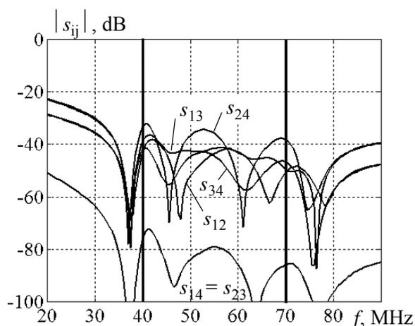
Fig.12. Characteristics of elements of scattering matrix of the antenna array with four-channel phase commutator and matching devices
