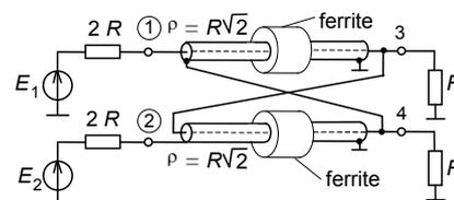
Fig.2. Structure of the cable hybrid (balun)
