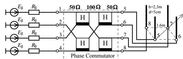
Fig.9. Structure of 4-port antenna array with four-channel phase commutator - uncoupler
