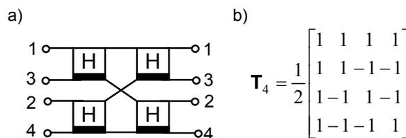
Fig.4. Structure (a) and transmission matrix (b) of 4-channel phase commutator
