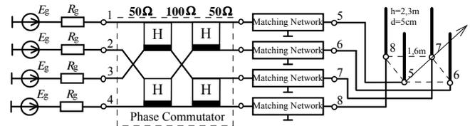
Fig.11. Structure of 4-port antenna array with four-channel phase commutator and matching devices
