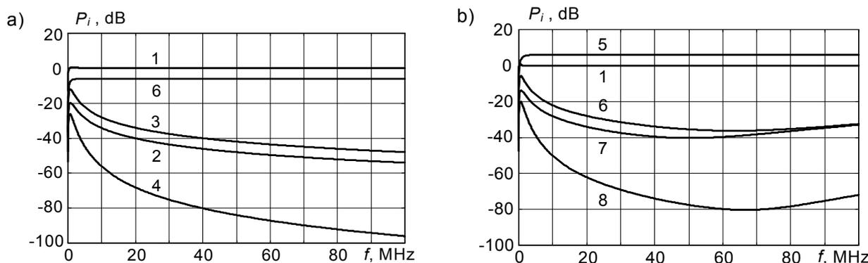
Fig.6. Frequency characteristics of the four-channel phase commutator with dividing (a) and summing of the power (b); matched loads
