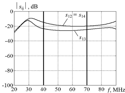
Fig.8. Characteristics of elements of scattering matrix of the antenna array
