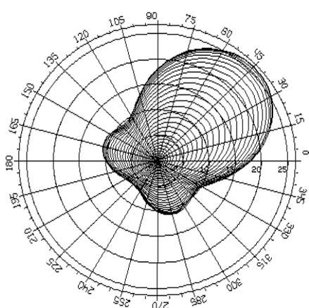
Fig.13. Characteristics of radiation of antenna arrays on 50MHz
