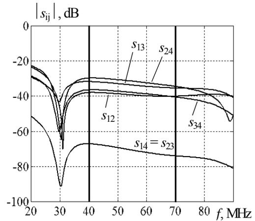
Fig.10. Characteristics of elements of scattering matrix of the antenna array with four-channel phase commutator
