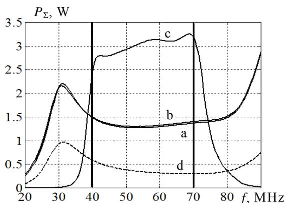
Fig.14. Characteristics of total power  $P_{\Sigma}$  radiation of the antenna array (a), antenna array with four-channel phase commutator (b) and antenna array with four-channel phase commutator matching devices (c), single antenna (d)
