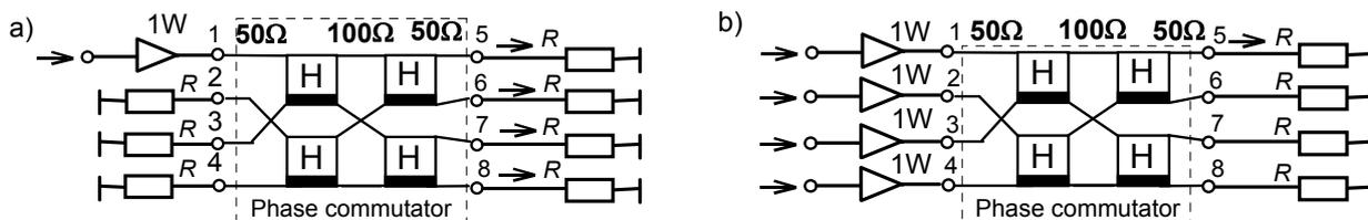
Fig.5. Structures of excitations of the four-channel phase commutator with dividing (a) and summing (b) of the power; matched loads
