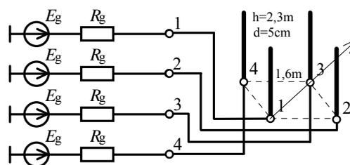
Fig.7. Structure and excitation of 4-port antenna array
