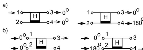
Fig.1. Principle of the hybrid operation: a) division of power, b) summing of power
