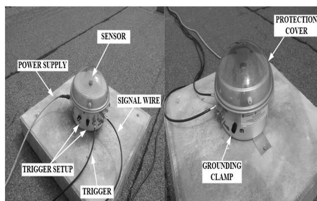
Fig.1. ELF-MF electric field sensor operating at the Lightning Research System of Rzeszow University of Technology
