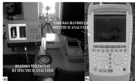
Fig.4. Spectrum analyzers used during calibration. a) RSA5106A RT Tektronix spectrum analyzer; b) FSH4 R&S handheld spectrum analyzer
